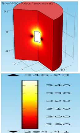
Fig: 6. Surface temperature of cylinder after 10 hrs.
